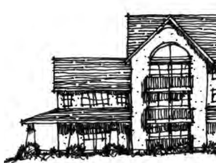
Taller buildings should be stepped back in height with the lowest towards the street or adjacent single-family homes.
