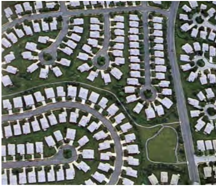
Subdivisions designed primarily with cul-de-sac decrease walkability and concentrate traffic on a few streets and intersections.
